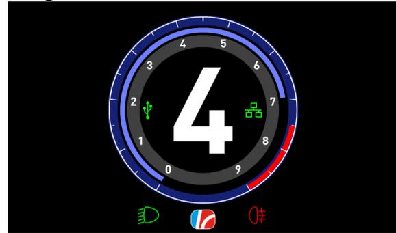
The Stage view is primarily for use in rally stages where a minimal display is often wanted. It displays the classic rev counter with a large gear number in the centre and optional text displays in each corner. Stage 2 has the same layout as stage 1 but with two monitoring items allowed in the centre. Stage 3 features the large gear number of stage 1 but also includes the bar gauges of road arrow. Stage Arc2 incorporates the alternative arc style.
