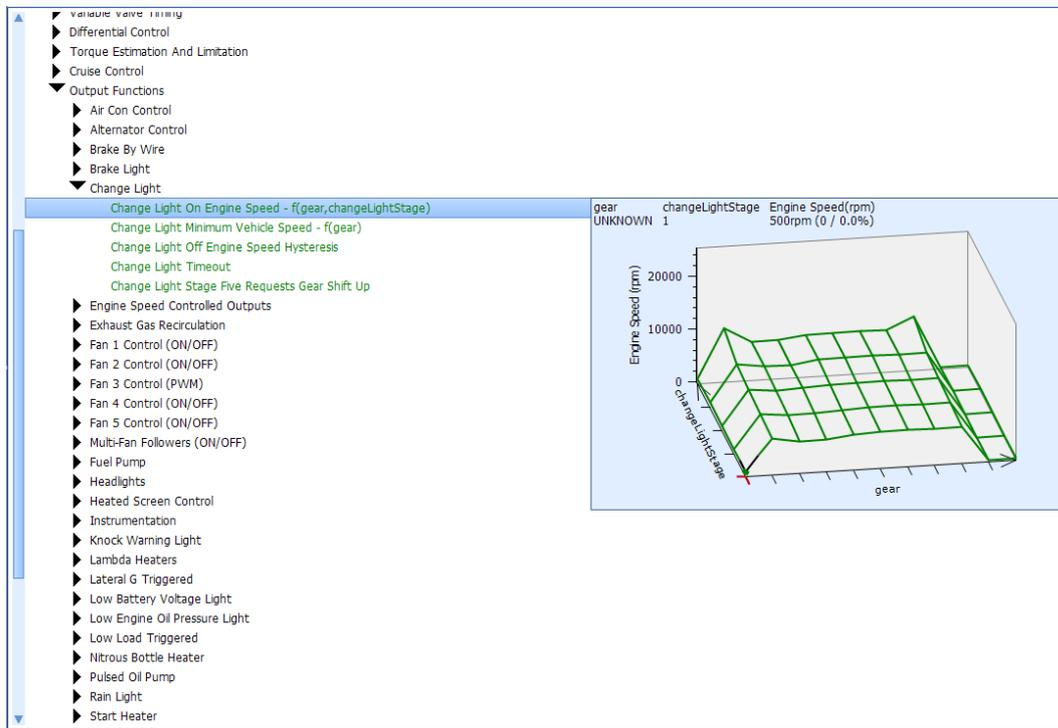
In *On Engine Speed – f(gear, ChangeLightStage)* each gear can have its shift light points independently assigned.
