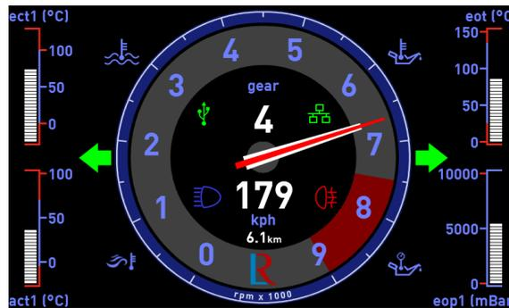
The Road templates display the classic rev counter with gear and speed located in the centre. There are also 4 gauges around the outside that can be set to display any numerical item. Common items also have a corresponding symbol. Road Arc and Road Arc2 use an arc rev counter and sweeping gauges in two different styles. Road Arrow uses a needle rev counter and bar gauges. The road pages are the only pages that display tell-tales such as indicators and lights.
