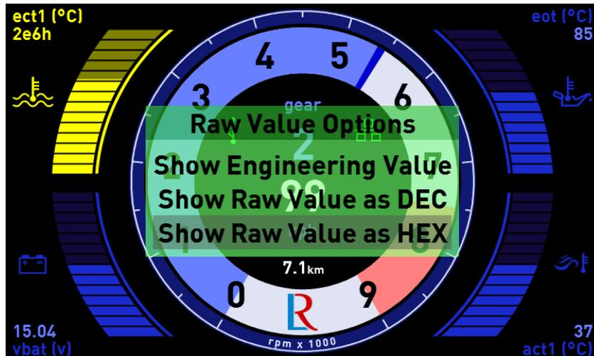
Most text gauges can also be viewed as a horizontal bar by enabling the option in the text menu. Alarm values will be displayed as vertical lines inside the gauge. When an alarm is triggered, the whole gauge will change to the alarm colour but the item value will appear yellow. The numerical value can be disabled so only the bar is visible if preferred.
