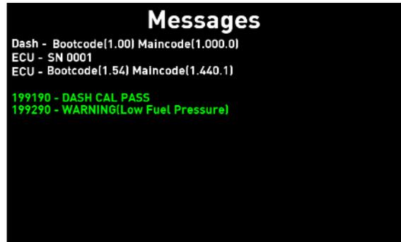
From dash v1.3.65 and ECU v1.661.1, these messages will be sent to the ECU and displayed in the ECUs messages during a live connection and added to the ECU logging. Acknowledgements will also be recorded.
