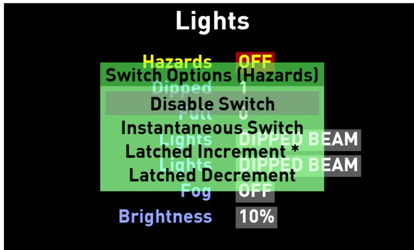
A selectable or switchable item will be distinguished by a surrounding box with the active item highlighted. Use the arrow keys to navigate.
