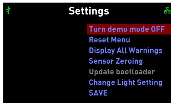
The settings page cannot be altered but gives some global options including input zeroing, lap stats reset and change light settings. The settings page is required to store any changes made on the dash itself.
