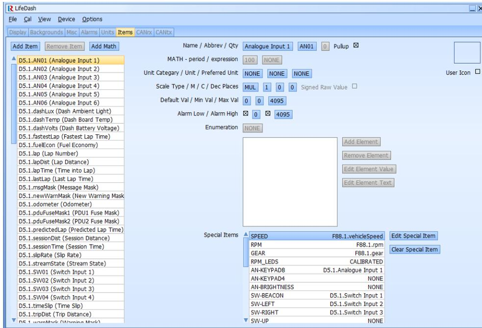
LR items are automatically added when an .LRC file is loaded in the 'CANrx' tab. Other devices must be added manually using the Add Item button and following the dialogue boxes. The dash will also have several of its own monitoring items including lap data and independent inputs. Lap data is calculated live in the dash as long as special items are defined and a lap beacon is connected. It also has its own items for dash voltage, temperature and ambient light sensor.
