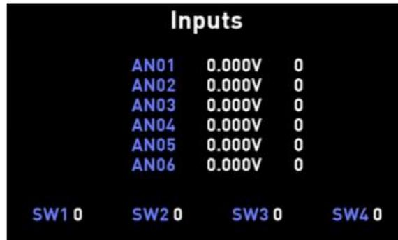
The inputs page displays the status of all the dash inputs. It can be used for input diagnostics and fine tuning linearisation. **This page cannot be edited.**
