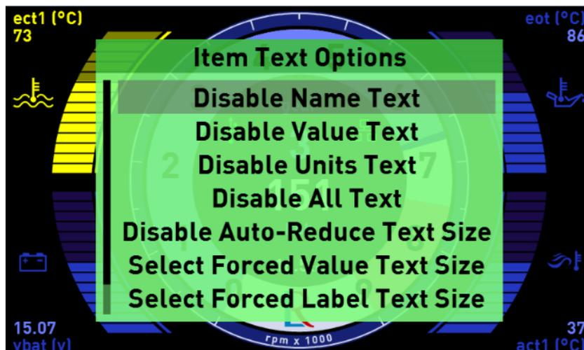
Also available is the option to display raw values rather than the converted engineering value. This can be used to diagnose faults and assist in correct CAN and item setup.
