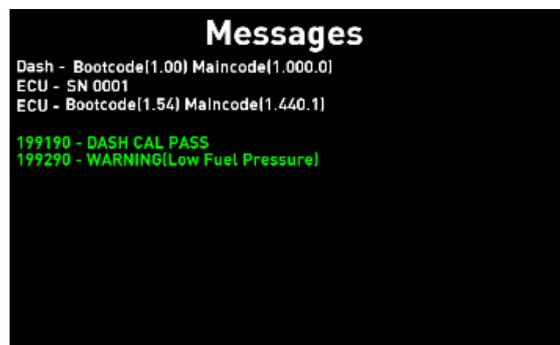
The message screen is used to display Dash and ECU information such as version and software levels, as well as any alarms that have been triggered. **This page cannot be edited.**
