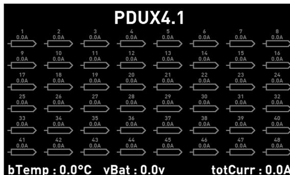
Intended for use with any Life Racing PDU, these pages will give current ratings and status of all PDU outputs and will automatically work when PDU items are added. Output abbreviated names will be displayed in place of the output number where available. Up to 2 of each type of PDU is supported. **These pages cannot be edited.**
