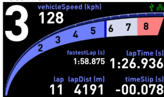
The Race Arc template uses a swept rev counter, a large gear indicator and several text displayers. The layout and number of text displayers differs from Race Arc1 and Race Arc2 depending on preference.
