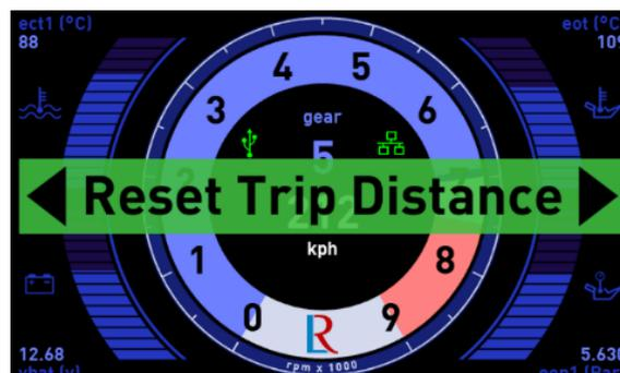
With Demo mode disabled, gauges will display default values set from the 'items' tab. The item values can be temporarily changed to a set figure using the **Set MonItem Values** button. This can be used to test alarm conditions, custom LED's and shift lights.
