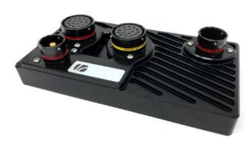
The PDU34A includes many of the features of the PDUXB range but in a smaller, lightweight package with Deutsch Autosport connectors for harsh environments where weight is paramount. The PDU34 has 16 inputs and 34 outputs. All inputs and 14 outputs can be slaved to an LR ECU. It is also sleep capable and includes 3x CAN 2.0b buses, 1x LIN (custom projects) and two port Ethernet.
