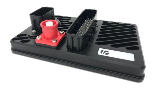
**Inputs** - Flexible input channels capable of support 0-5v, thermistor, bi-polar and frequency type signals
