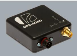
The Life Racing GPS-AG50 is a compact low mass unit capable of tracking vehicle speed by GPS position at 50Hz. The unit features a built-in 6-axis motion pack for measuring lateral, longitudinal and vertical acceleration as well as roll, pitch and yaw rates. The module connects to any device via the CAN network.
