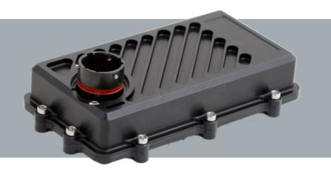
Life Racing's direct injector driver is a compact unit capable of driving four fuel injectors at a high voltage, thus catering for the requirements of high-pressure solenoid injectors. The unit generates the complex waveforms required to activate the injectors. The injectors are switched on via pulses from the host ECU.
